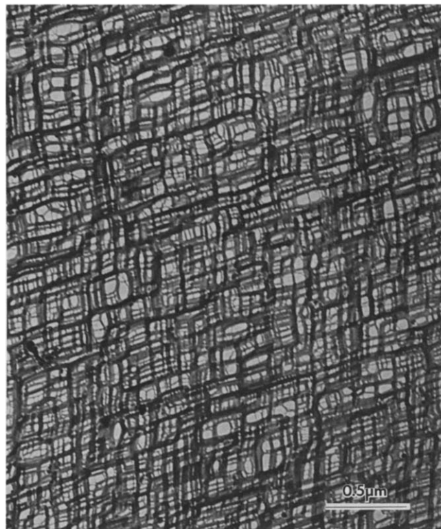
Figure 1 Electron micrograph of polyacetylene polymerized epitaxially on the substrate crystal of terphenyl at -78^{\circ}\text{C}
